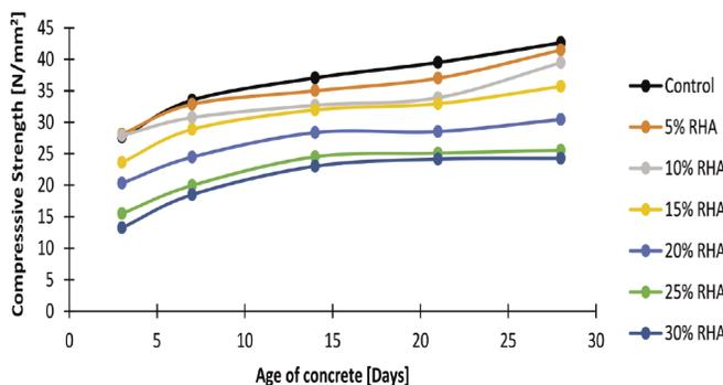
Fig. 4 Compressive strength result at different RHA replacement levels
