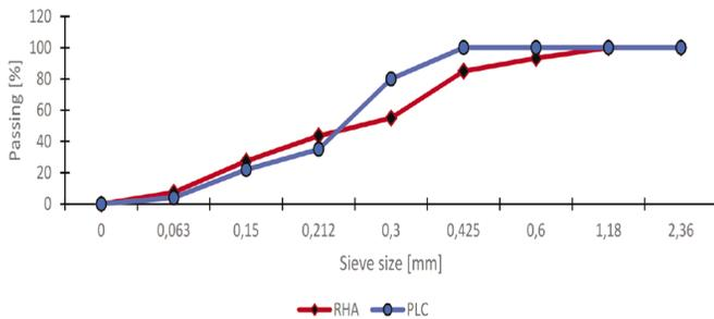
Fig. 3 Particle size distribution for RHA and PLC
