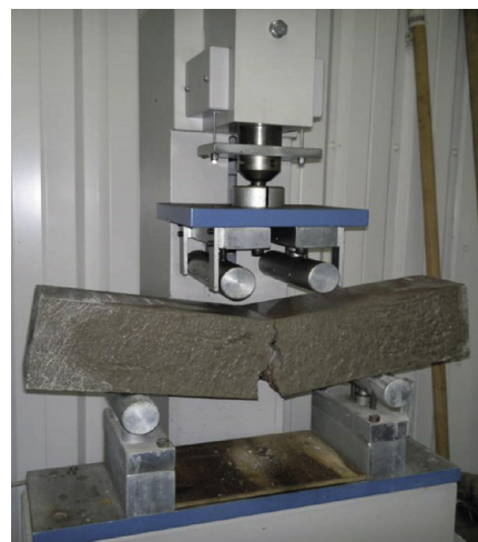
Fig. 11 Flexural strength apparatus
